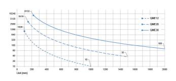
sible load based on a shaft deflection of 1/1000 of Ltot. For long units, actual load may need to be reduced to achive a deflection acceptable for the application
