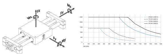
\*All capacity values are theorethical maximal values without any safety factor.
